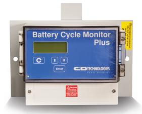
The Battery Cycle Monitor Plus (BCM 2200-NM) continuously monitors the most critical performance characteristics of the battery system: string voltage, battery current, ambient temperature, quantity and duration of discharges.
