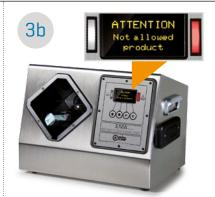
If the container content is not conforming, a YELLOW or RED light and an **ALARM message** ["Not allowed product"] are displayed.
