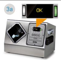
If the container content is identified as conforming, the "OK" message and a green light are displayed.
