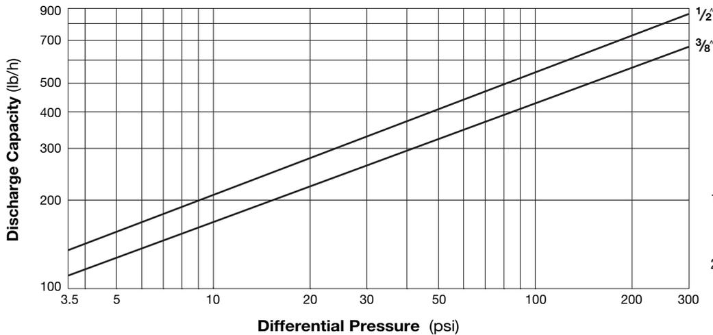
1. Differential pressure is the difference between the inlet and outlet pressure of the trap.
