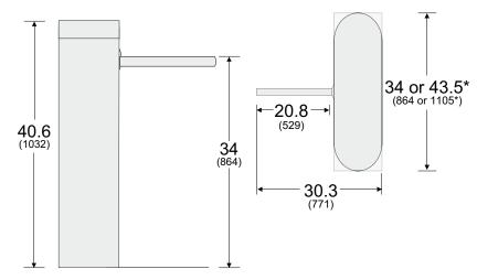
\* Width of EDC-EBN Dimensions shown in inches (mm). All Measurements are approximate.
