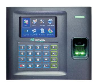
CronoStation is a versatile solution for T&A and access control which combine a highly durable yet elegant casing with a variety of identification methods from barcode cards, to fingerprints and 125 kHz, Mifare or HID iClass proximity cards.
