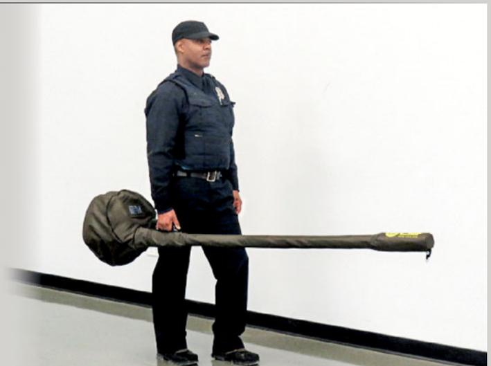
The **CEIA MSD** is a one-piece, portable and full-height ferromagnetic detector that **combines high reliability and ergonomics with advanced detection** and operator signaling features.
