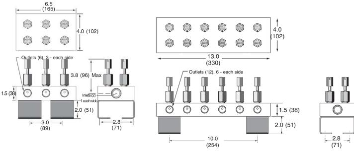
Weight: 13 lbs (5,9 kgs) Orifice Size: 0.19" Weight: 24 lbs (10,9 kgs) Orifice Size: 0.19"
