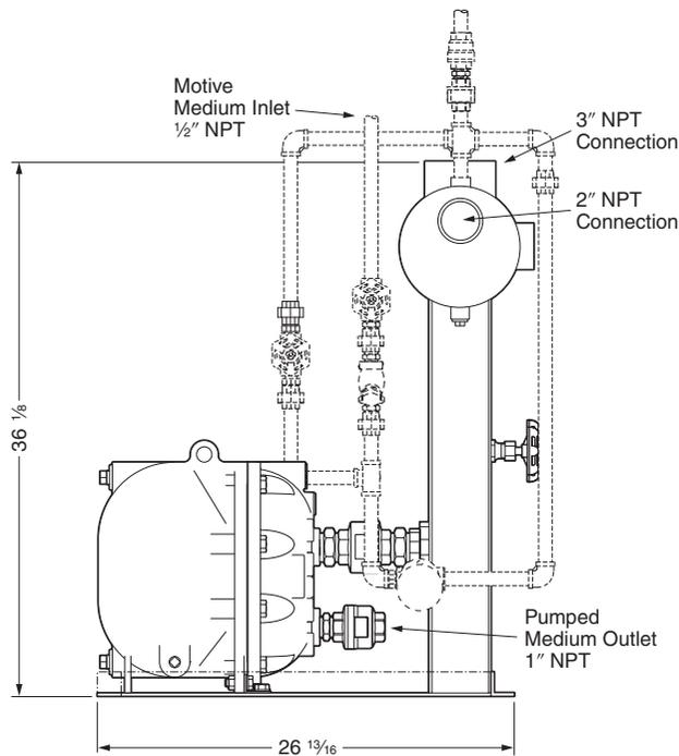
**NOTE:** Piping and valves indicated by dashed lines can be provided at an additional cost.
