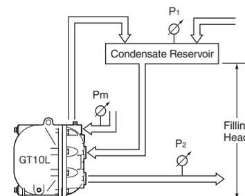
The discharge capacity is determined by the motive medium, motive medium pressure (P<sub>m</sub>) and back pressure (P<sub>2</sub>).
