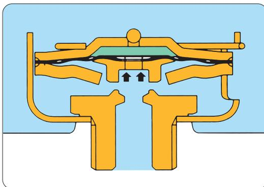
During start-up of steam using equipment, steam mains, or tracers, the fill is in the liquid state while the capsule is still cold. While the fill is liquid, the internal chamber pressure is lower than the external primary pressure. This difference allows the diaphragms to be raised by the external pressure and open the valve so that air, other incondensibles and condensate can be discharged.
