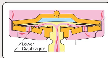
When the lower diaphragms suffer only a slight tear and the valve head is intact, the trap may leak, but it can still discharge condensate at the maximum discharge rate.
