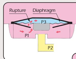
1. When the diaphragm attached to the valve head breaks, its liquid fill escapes. This allows the primary pressure, P1 to build up in the chamber above the diaphragm.
