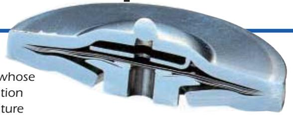
The "X-element" internal chamber contains a liquid fill whose saturation temperature is slightly lower than the saturation temperature of water. With rising condensate temperature reaching the trap, the fill evaporates and its resulting internal pressure expands the diaphragms to close the valve. When the condensate temperature cools, the fill condenses and its resulting pressure reduces allowing the diaphragms to contract for the valve to open.
