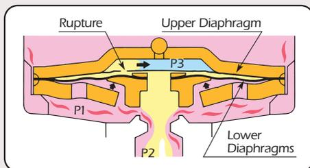
The internal chamber pressure "P3", equalizes with the downstream pressure, "P2". This causes the lower diaphragms and attached valve head to be lifted by the primary pressure, "P1", which opens the valve.
