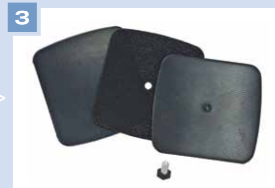
3 EPDM raw material prepared for vulcanisation – between two EPDM sheets there is a layer of re-enforcement material.
