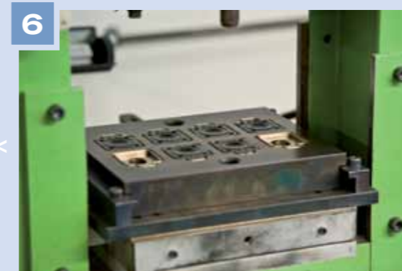
6 After completion of the vulcanisation process the completed diaphragms can be removed from the tool.
