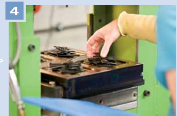
4 The vulcanisation tool on the press – the EPDM blanks are placed in the moulds.
