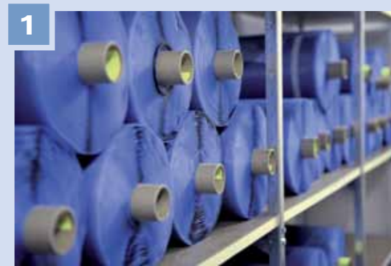
1 The raw material is stored in an air conditioned warehouse that is protected against light. This enables less alteration of the material.
