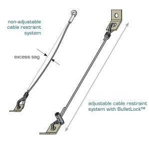
Installing cable restraints can be a physically gruelling exercise. The installer often needs to install seismic cable restraints in hard to reach areas to restrain ductwork and piping. The challenge is compounded if the restraint system is not adjustable because crimping requires considerable physical effort and an adequate amount of space to operate the crimping tool.
