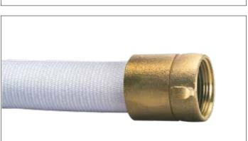
This **SINGLE JACKET FIRE HOSE** has a proof test pressure of 500 psi and a service test of 250 psi. It features 100% polyester rubber-lined material for extra strength and flexibility. FM approved. **NOTE:** Recommended for industrial fire protection.
