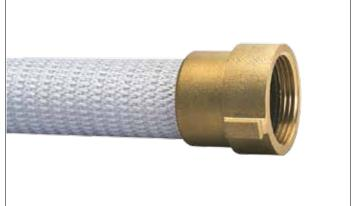
For emergency use only, this **PACK & REEL FIRE HOSE** is fully lined and FM approved. It has a proof test pressure of 500 psi, service test of 250 psi, and comes folded for easy installation on pin racks. Brass NST coupled.
