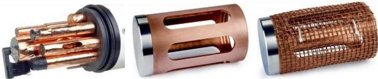
This document provides guidance for effective use of copper as an anti-fouling tool for Hydrolab sondes and covers the application of copper tape, sonde guard, and mesh.
