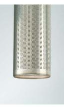
Power VT Plus uses a stainless steel pre-mix surface burner enabling low NOx operation. A zero-governor gas valve provides for infinitely proportional mixing of gas and air, assuring proper combustion under all vent pressure conditions. A combination natural gas and LP gas train is available for backup fuel utilization.
