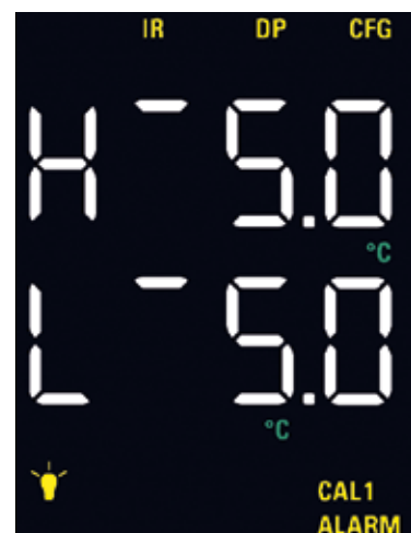
Dew point alarm configuration
