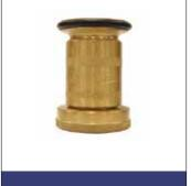
INDUSTRIAL WASHDOWN NOZZLES come standard with variable streams (shut off, straight stream, and fog). 100 psi max operating pressure. Satin brass finish.
