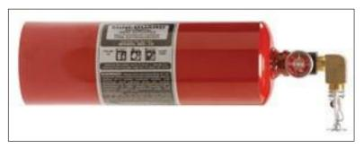
The Mini-Guard automatic spot protection extinguishers are designed, constructed, and tested to the same engineering standards as our portable fire extinguishers. Available in horizontal or vertical configurations, the units can be charged with multipurpose (ABC) dry chemical or Halotron agents and are fitted with a detection sprinkler head that is rated at 165° F.
