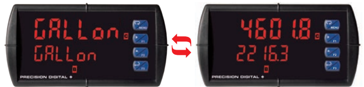
Lower Display Alternating Input Channels A & B
