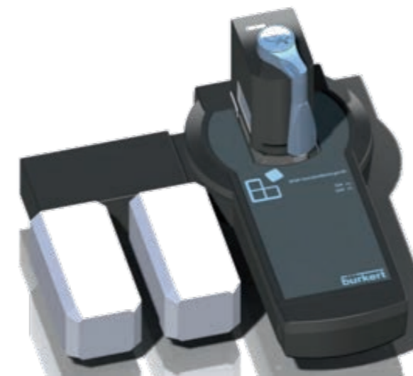
Handheld calibration unit Type MZ15: Calibration can be done by plugging in the right calibration buffer and the Sensor Cube. Operation is controlled via a connected Bürkert Communicator or a Type 8905 system with 7" touch display.
