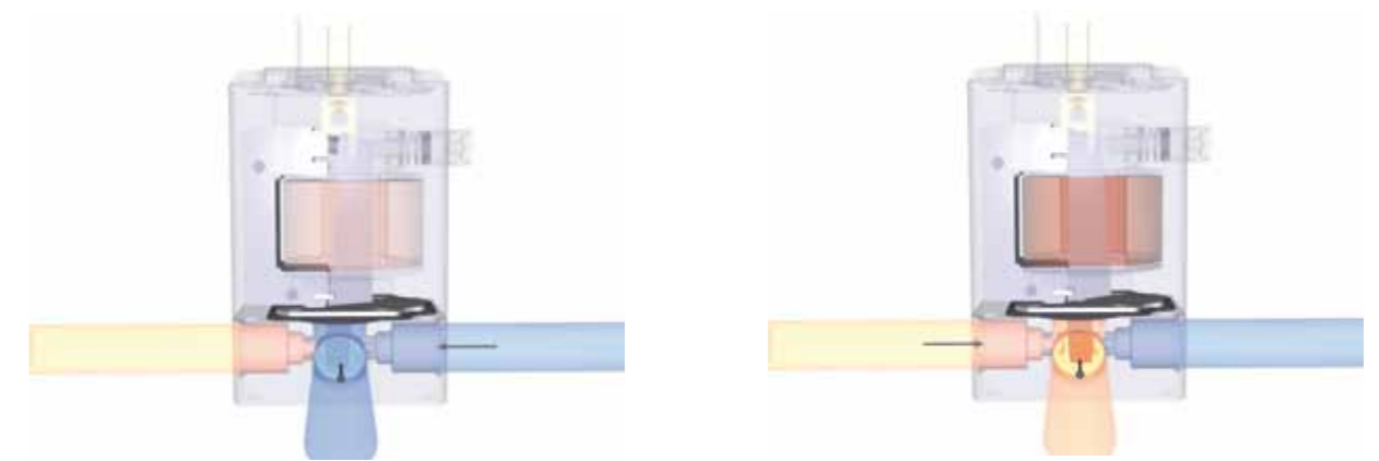
Operating principle of the 3/2-way pivoted armature valve with standard media separation and manual actuation
