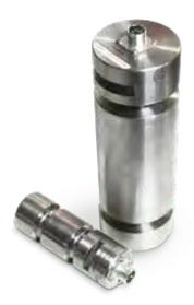
A key component for MSI's integrated overhead weighing solutions is the Load Pin Sensor. Typically designed and manufactured specifically to each integrated solution, the MSI load pin is strictly industrial grade. Each load pin design is precision machined from 17-4 stainless steel for safety, strength and corrosion resistance.
