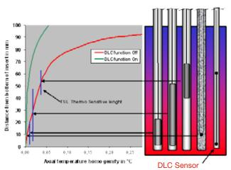
Axial temperature curves for an RTC calibrator with and without the DLC functionality activated. DLC controlling is automatically disabled when the stirrer is started.
