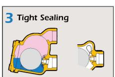
When the flow of condensate stops, the float seats on the orifice supported by the orifice and two machined guides. The water level remains above the orifice to provide a steam-tight seal. The temperature keeps the bimetal retracted so that it does not affect the float's seating.
