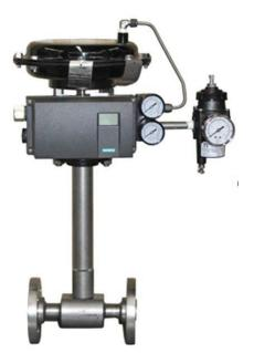
Mark 8000 in Inconel 625 with ANSI 300 Flanges, extended bonnet and Mark 16IQ Smart Positioner The Mark 8000 provides incredible flexibility in a control valve often used in critical applications, where service or environmental conditions may be too harsh for traditional lighter-duty fractional flow valves. The barstock construction allows us to provide materials appropriate for most applications while meeting aggressive delivery requirements.
