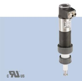
pH transmitter with programmable outputs. pH and temperature output via single or dual analog 4-20 mA. Two transistor outputs are also included. Transmitters are engineered for a wide scope of measuring ranges and can be delivered in 2-wire or 3-wire configurations. Intelligent, integrated, beautiful design fits perfectly with an assortment of easily configured fittings.
