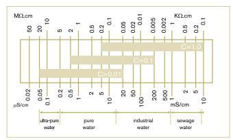
The electrode is selected according to the measuring range and medium by using this table.
