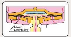
When the lower diaphragms suffer only a slight tear and the valve head is intact, the trap may leak, but it can still discharge condensate at the maximum discharge rate.
