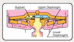
The internal chamber pressure "P3", equalizes with the downstream pressure, "P2". This causes the lower diaphragms and attached valve head to be lifted by the primary pressure, "P1", which opens the valve.
