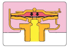
High condensate temperature evaporates the "X-element" fill and increases the internal chamber pressure to expand the diaphragms.
