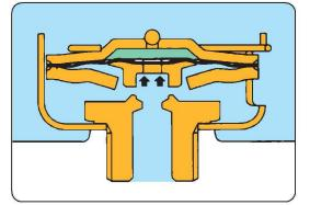
During start-up of steam using equipment, steam mains, or tracers, the fill is in the liquid state while the capsule is still cold. While the fill is liquid, the internal chamber pressure is lower than the external primary pressure. This difference allows the diaphragms to be raised by the external pressure and open the valve so that air, other incondensibles and condensate can be discharged.
