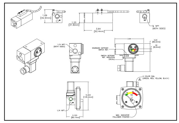
**TEMPERATURE LIMITS:** -40 F (-40 C) to 200 F (93 C). These limits are based on the entire instrument being saturated to these temperatures. System (process) temperatures may exceed these limitations with proper installation. Contact our customer service representative for details.
