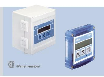
Unique batch controller for accurate filling of liquids. This universal IP65 controller is wall mounted and compatible with all sensors with an open collector pulse, relay reed, TTL, CMOS or coil output.
