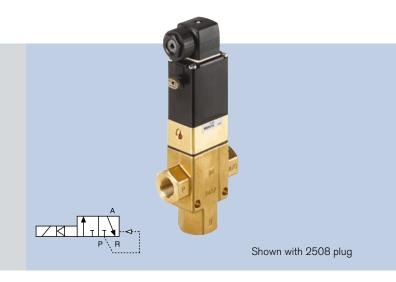
Servo-assisted 3/2 way normally closed and normally open solenoid valve with a pivoted armature and isolating diaphragm. This series encompasses a range of diaphragms, sealing materials and electrical connections. Perfect for pneumatic actuation of very large process valves.
