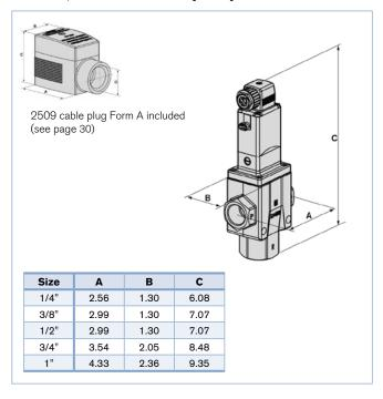
Port connection Orifice Cv Item no. Voltage/Frequency [V/Hz] Pressure range [inch] [mm] [PSI] 24 V DC 24 V/60 Hz 120 V/60 Hz **Circuit function C** NPT 1/4 8 1.1 7-232 453 286 98101599 \_ NPT 3/8 2.7 7-232 12 453 378 NPT 1/2 12 3.0 7-232 453 290 453 291 453 292 NPT 3/4 20 7.7 7-232 98100981 464 358 453 296 NPT 1 25 11.7 7-232 461 657 453 300 \_ **Circuit function D** NPT 3/8 12 2.7 7-232 \_ 454 091 \_ NPT 1/2 12 3.0 7-232 453 310 \_ 453 312
