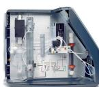
Strategy A: used in membrane conductometric methods, which calculate TOC = TC - IC
