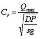
From the Cv chart on Page 2, pick the smallest valve that has at least the Cv determined above, and where the velocity does not exceed 25 ft/sec.
