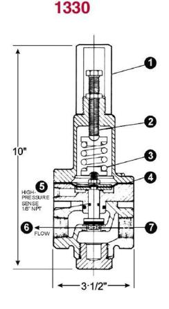
Pilot Materials Bronze B-61 Stainless Steel ASTM A743/CF8M
