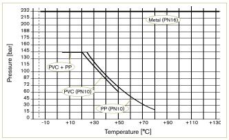
Note: Always take lowest Max. medium temp. of both adapter and used ELEMENT transmitter.
