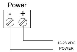
**Figure 2. Power Connections**
