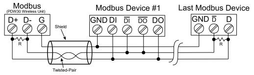
Figure 8. Multiple Device RS-485 Modbus Connection
