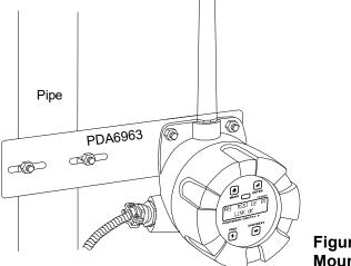
Figure 11. PDA6963 Stainless Steel Pipe Mounting Kit
