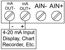
Figure 5. 4-20 mA Output Connections
