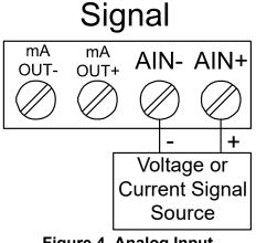
Figure 4. Analog Input Connections
