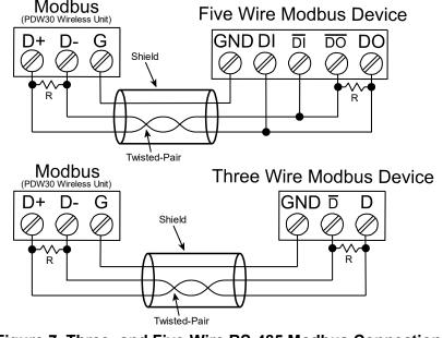
Figure 7. Three- and Five-Wire RS-485 Modbus Connections
