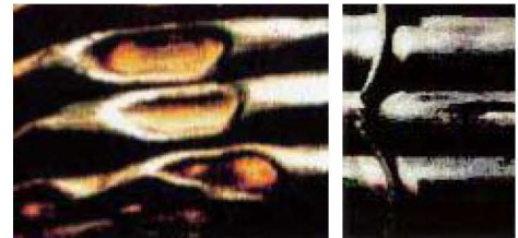
Water hammer damage to tubes and stays
