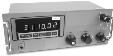
DLR3110 - 19 inch wide rack-mountable version of DLR334 plus precision patented Orion valve assembly and vernier, test port and test hose, pressure limit control and monitor.*** Test port may be mounted on front or rear of unit *** Pressure limit control and monitor are not required for 5000 psi models and above
