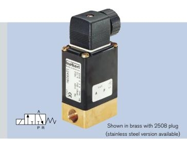
Direct-acting 3/2 way normally closed and normally open solenoid valves with pivoted armature and isolating diaphragm. This flexible valve series includes many options, various body materials, diaphragm and sealing materials and a range of electrical connections to suit many applications.
