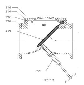
Shown with optional backflushing actuator
