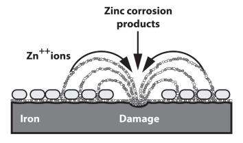
Zinc is anodic to iron. That means iron is the more stable, more noble, of the two elements. Zinc will cathodically protect the iron pipe as long as zinc is present, and over time, will convert to zinc compounds that provide an enduring passivating layer under the topcoat, which protects the pipe against further corrosive attack. Zinc is an anode, uniformly adhered to the surface of the pipe.
