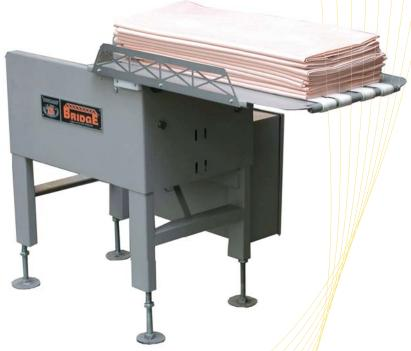
The Bridge linen transition conveyor neatly transfers stacks of folded linen from a large piece or towel folder onto a master linen conveyor system. After receiving stacked linen directly from a folder's discharge conveyor, the Bridge's motor-driven roll advances the stack across its heavy duty mini-conveyor.
