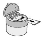
Lift the lid. Using a small screwdriver blade, carefully remove the pulser clip
