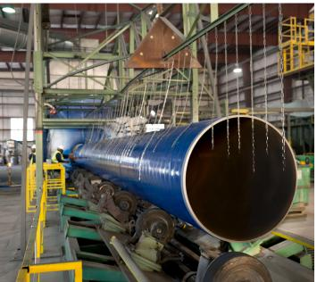
Polyurethane coating meeting the requirements of ANSI/AWWA C222 is available from AMERICAN. Polyurethane coating is typically applied at 25 mils minimum DFT, but thicker coating is possible.Contact an AMERICAN representative regarding increased coating thickness. The coating is applied and tested for conformance as described previously for polyurethane lining.
