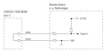
Whenever a pulse is generated, the electronic switch at the DFM 8EDM will be closed and the incoming 12-24VDC will be redirected to the external device.
