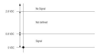
Below  $0.8\ VDC = pulse\ (logic\ 0)$ Between  $0.8-2.8\ VDC$  is not defined Over  $2.8\ VDC = no\ pulse\ (logic\ 1)$
