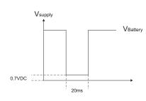
Whenever a pulse is generated, the electronic switch at the DFM 8ECO will be closed and the incoming 12-24VDC will be redirected to the external device.
