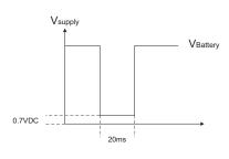
Whenever a pulse is generated, the electronic switch at the DFM 12ECO will be closed and the incoming 12-24VDC will be redirected to the external device.
