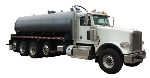
This spiral-wound, robotically welded, 1/4" material protects against the most corrosive environments and materials. Every ARM vacuum system is equipped with an interior tank lining for superior corrosive protection.
