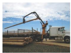
The lightweight design of the ELITE series, combined with an incredible 8,770lb (910)/10,960 (915) lbs max lift capacity make these two loaders the undisputed heavyweight champions in their weight class. Lift more with less than you ever imagined.
