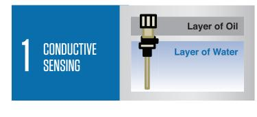
Stancor's patented technology on conductive sensing, which measures the electrical current in a liquid and has proven to reliably differentiate oil and water, has been applied to a field base of more than 25,000 systems. Self-cleaning, conductivity probes are maintenance-free compared to optical sensors that attract contaminants.
