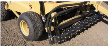
For the models Cherrington 4600 XL and 440 XL we offer an optional pre-screening powered roller for soil preparation. This truly makes this maschine a one-step seedbed prep tool. The hydraulically powered roller with hydraulic depth control is an
