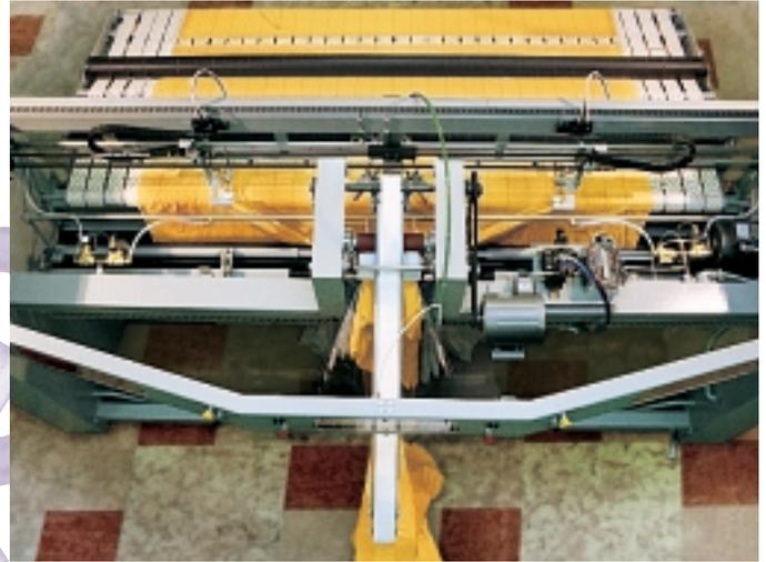
The ability to handle several pieces sequentially within the system at the same time and a maximum cycle rate in excess of 1200 per hour means that the Edge can deliver a consistently high volume of work to high speed ironers with fewer operators than any other feeding system.
