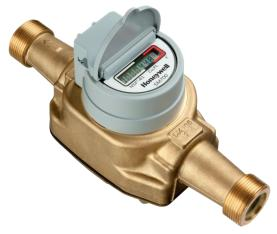
The oscillation is monitored by electrodes placed next to each diffuser wall, in which an electrical current is induced in the jet by a pair of powerful permanent magnets. Sensing electronics capture when the oscillations occur and totalize the volume passed displaying the registered volume on a liquid crystal display.
