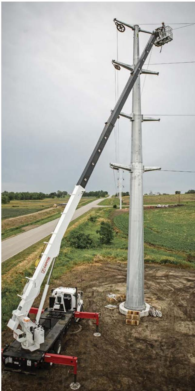
Boom trucks can be optionally equipped with work platforms that enable them to position people<sup>1</sup> in addition to lifting loads. With an Elliott boom truck, work platforms come standard with a two-person detachable gravity-leveled steel basket with a hydraulic lifting system. Range diagrams and load charts can be found inside the basket for quick reference.
